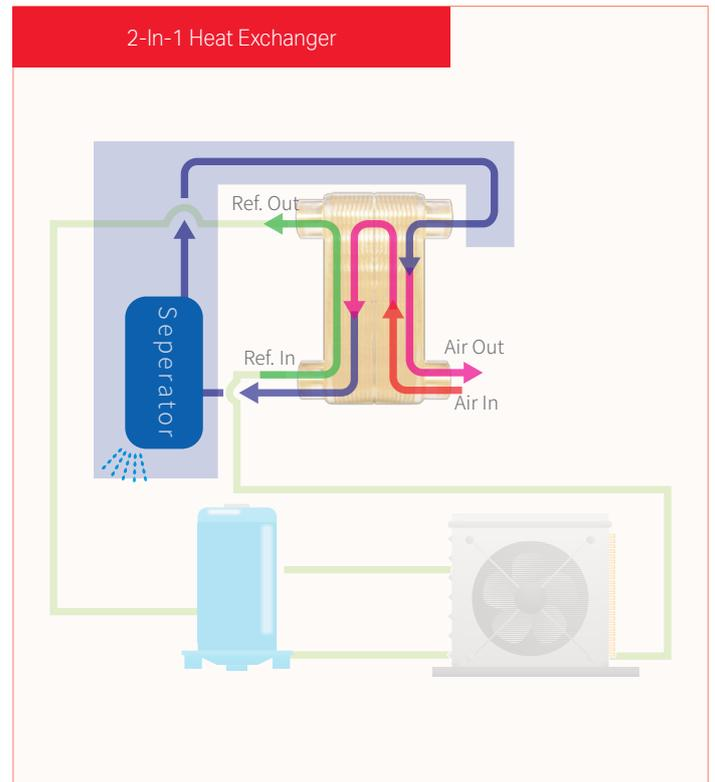
KAORI A series is an easy tubing heat exchanger which combined with a separator, as long as you connect the air inlet/outlet connectors, it's ready for use in your operation.
