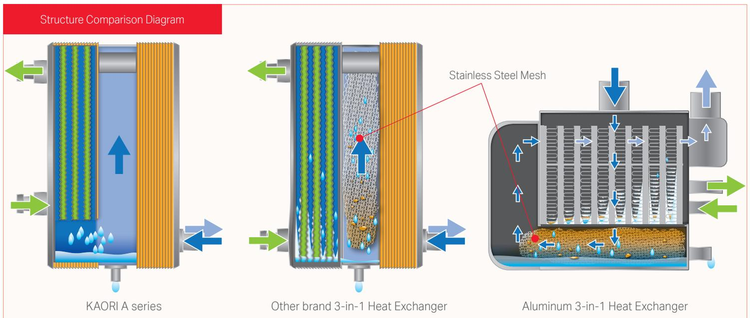
With KAORI exclusive designed separator, moisture and compressed air are effectively separated by gravity and centrifugal force, with exclusive non-mesh design could efficiently avoid the ice or oil clogging problems and extend the usage life.
