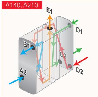
For the application using cascading refrigerated and desiccant dryers, Kaori's D Type adopts a new flow path design that directs the chilled dry air from the gas-water separator into the desiccant dryer for deep dehumidifications. After reaching the dew point temperature of -40~-94 °F, the air then returns to the D Type for use after preheating.
