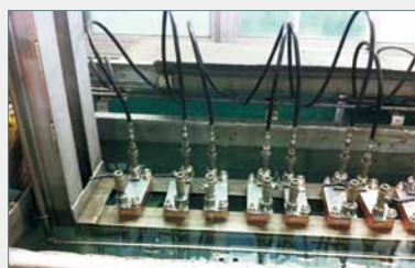
Pressure Leakage Test
