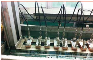
Pressure Leakage Test
