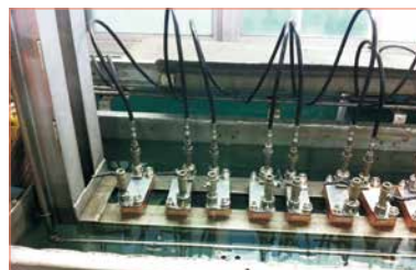
Pressure Leakage Test
