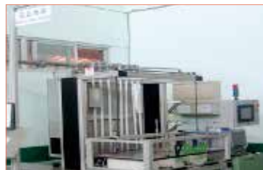
Helium Leakage Test
