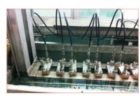
Pressure Leakage Test
