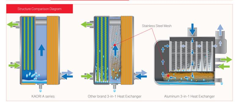
With KAORI exclusive designed separator, moisture and compressed air are effectively separated by gravity and centrifugal force, with exclusive non-mesh design could efficiently avoid the ice or oil clogging problems and extend the usage life.
