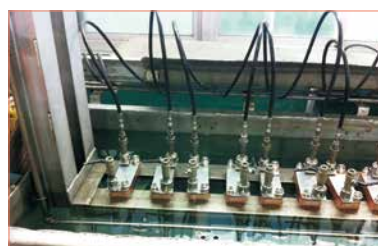
Pressure Leakage Test
