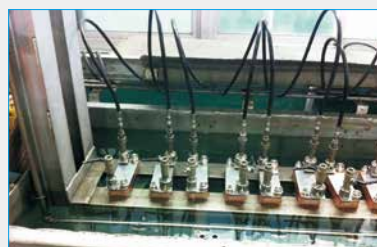
Pressure Leakage Test
