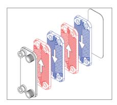
refrigerant leaves the condenser from the bottom left connector (A2). The water enters the condenser at bottom right (B2) and leaves the condenser from top right (B1). In the case of the condenser, heat is transferred from refrigerant to water and both fluids are in counter flow direction.
